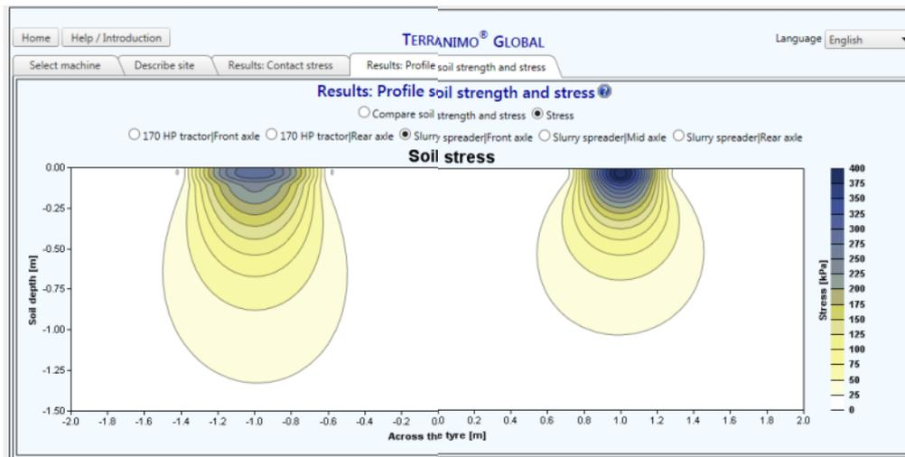
Figure 7. Terranimo-predicted stress distribution in the soil profile below a similarly loaded and inflated implement tyre at field capacity water content (left) and at the wilting point (right).
