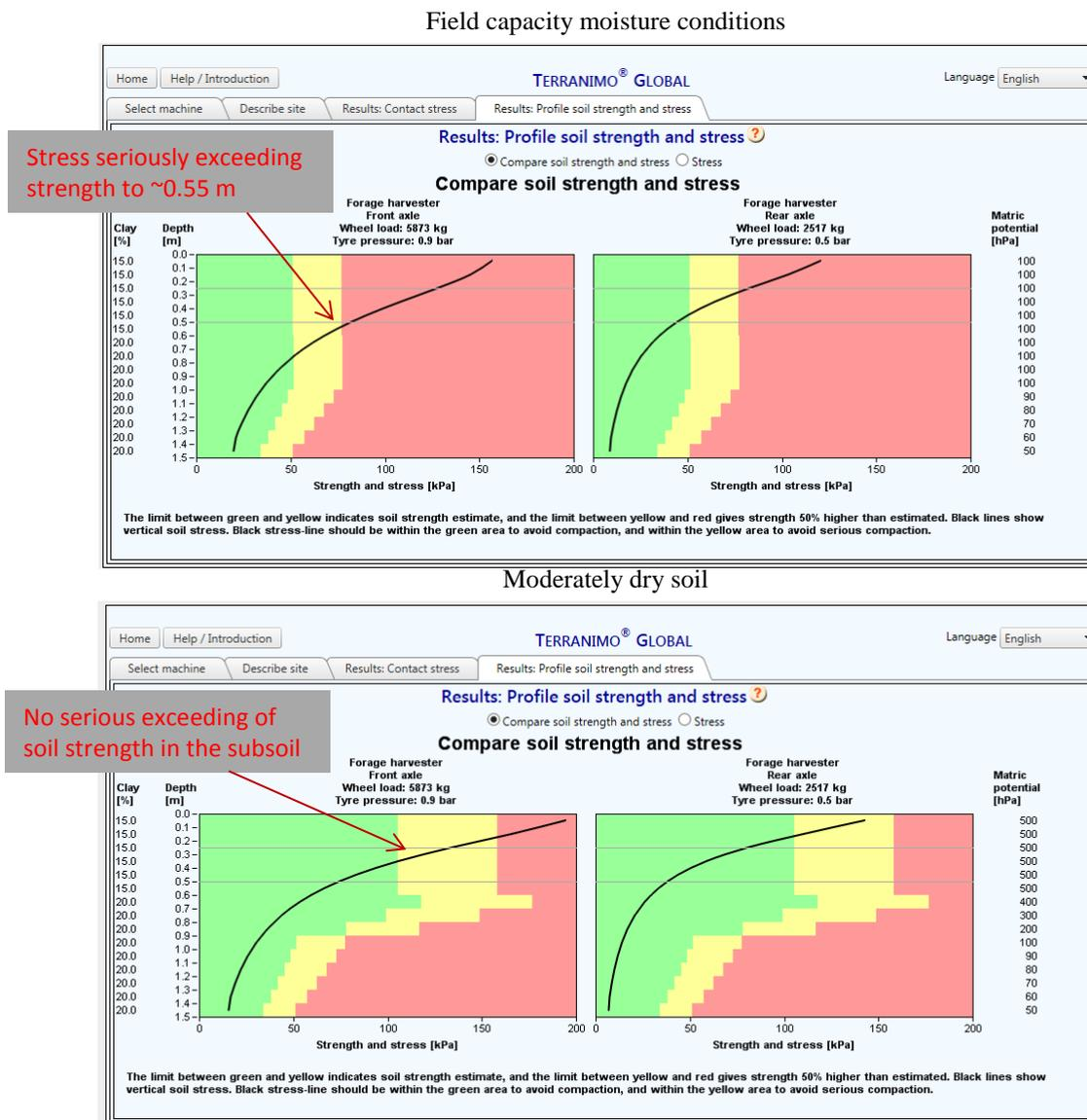
Figure 4. Comparison of stress and strength for the front and rear tyres of a forage harvester driving on a silty loam soil at field capacity moisture conditions (top) or when the soil is moderately dry (bottom).
