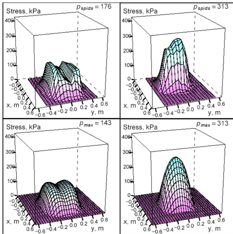
Figure 5. Measured vertical stress at the tyre-soil interface (upper part-Figures) and FRIDA-modelled stress-distribution (lower-part Figures). The data derives from a Michelin Cargobib 650/65R30.5 implement tyre loaded with ~60 kN (~6 tonnes) and either the recommended 1.0 bar (left) or 2.4 bar (right) inflation pressure. Data from Schjønning et al. (2006).
