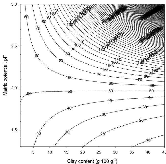
Figure 5. Estimates of soil strength (kPa) used in Terranimo<sup>®</sup> International as influenced by soil content of clay and the matric potential, expressed here as pF (small values: wet soil; high values: dry soil). Note that the strength estimates are regression-predicted based on measured precompression stress values scaled to yield 50 kPa at pF2.
