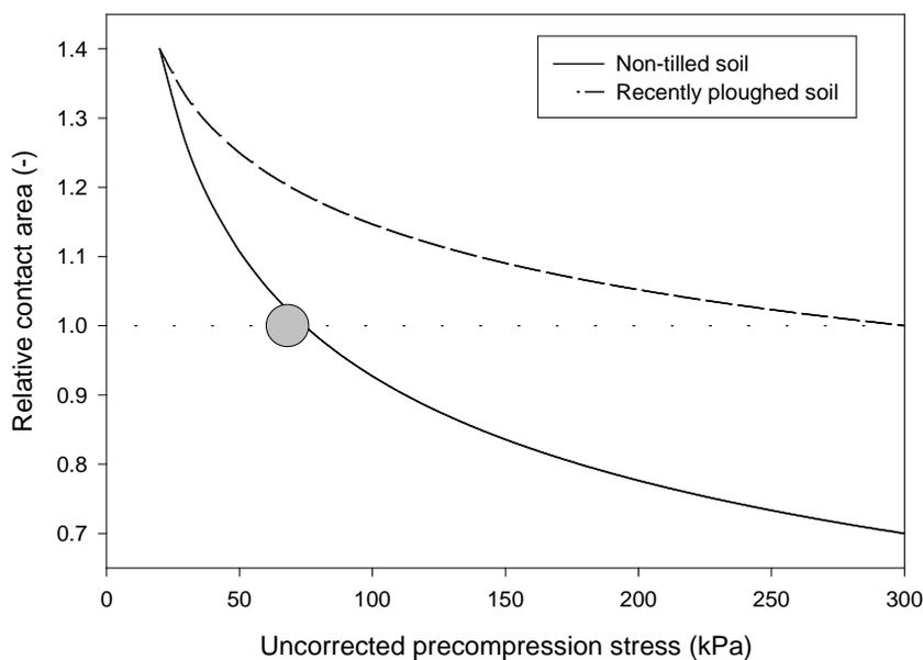
Figure 6. Terranimo<sup>®</sup> prediction of topsoil strength effects on the tyre-soil contact area. The gray symbol represents the topsoil strength condition for the comprehensive data set (Schjønning et al., 2006) being the main data behind the equations for estimating FRIDA parameters in Terranimo<sup>®</sup> (Schjønning et al., 2015b).
